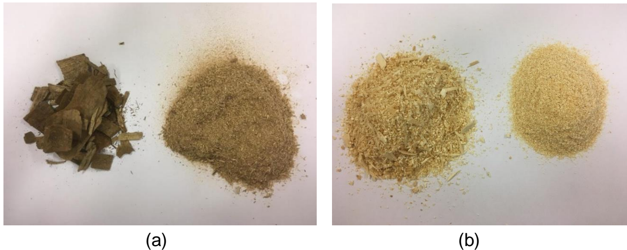
Figure 2. Wood chips (A) and sawdust (B) before and after grinding in a hammer mill
