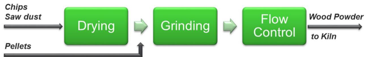
Figure 4. Block diagram for wood treatment before firing in kiln.
